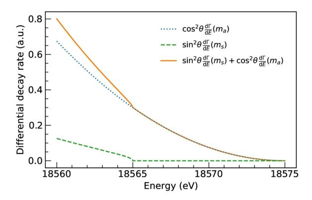
The results of the KATRIN experiment rule out a light sterile neutrino with a mass between 3 and 30 electronvolt. A neutrino within this range would have revealed itself by a bend in the orange line, e.g. as shown here at 10 electronvolt under the final value of 18.6 kiloelectronvolt. (Green line: Spectrum of a virtual light sterile neutrino with a mass of 10 eV; blue line: spectrum of the classical, active neutrino; orange line: combined spectrum. Credit: Plot: KATRIN collaboration
