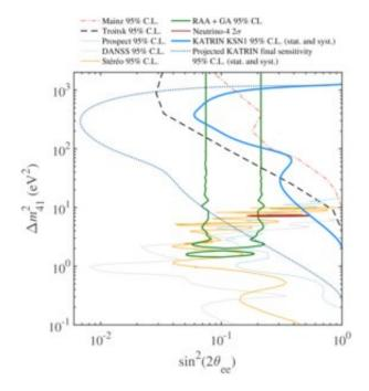
The area to the left of the lines shows the search ranges of the various experiments for the light sterile neutrino. The area inside the green lines marks the most likely location for light sterile neutrinos. Evaluations of the KATRIN experiment (blue solid line) significantly reduce this search range. Credit: Plot: KATRIN collaboration
