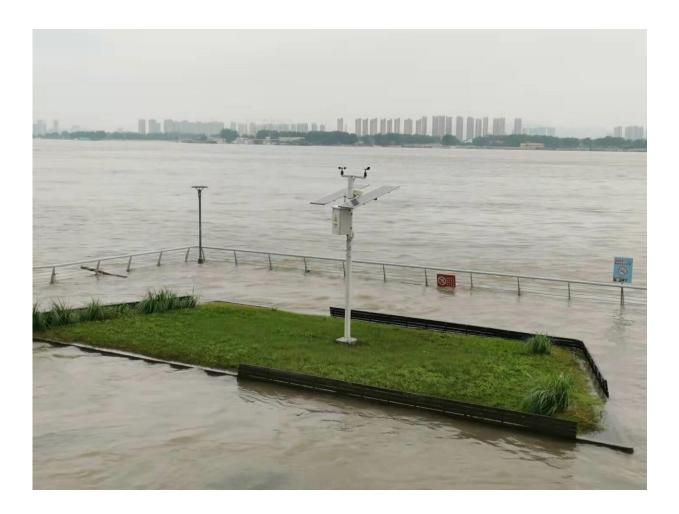
Automatic weather station near the Yangtze River in Nanjing, which flooded on 23 July 2020 Credit: Bing Zhou
