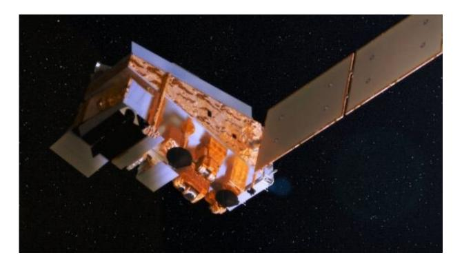
The Suomi NPP satellite which houses multiple instruments for imaging the Earth, including VIIRS. Credit: NASA
