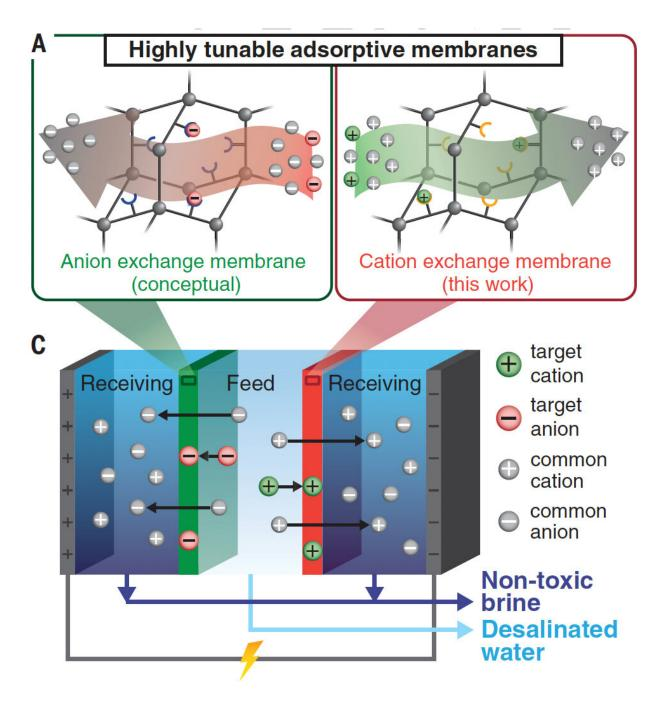
Polymer membranes with embedded nanoparticles that selectively remove ionic compounds (top) are employed in electrodialysis (bottom) to remove not only salt but also metals, many of which are toxic, producing pure clean water and a non-toxic brine that is easier to dispose of. The membranes (green and red) can be flushed and reused many times, while valuable metals could potentially be salvaged. Credit: UC Berkeley photo courtesy of Adam Uliana
