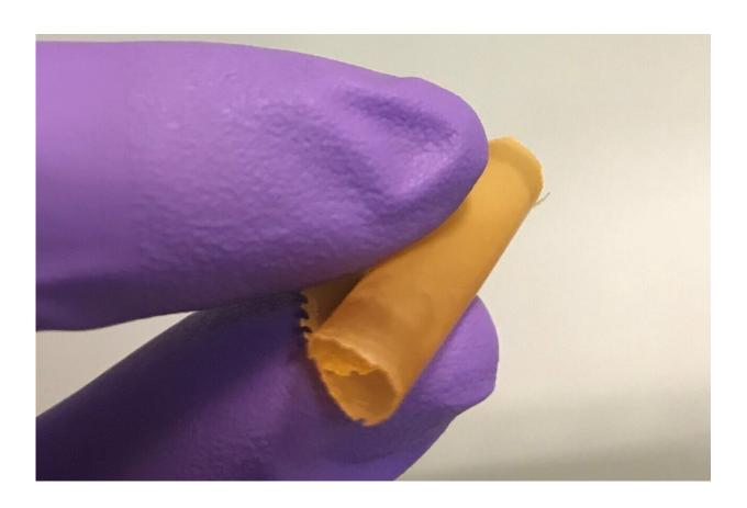
A flexible polymer membrane incorporating nanoparticles of PAF selectively absorbs nearly 100% of metals such mercury, copper or iron during desalination, more efficiently producing clean, safe water. Credit: UC Berkeley photos courtesy of Adam Uliana
