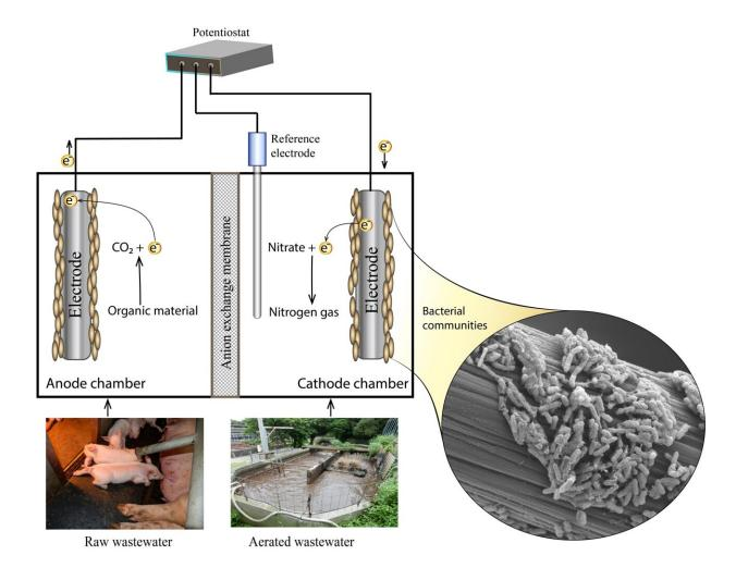
To treat both kinds of water, the researchers devised an ingenious solution; they used microbes to not only drive the treatment process, but also to recover some valuable nutrients out of the wastewater at the same time. The system was created from polyacrylic reactors containing two chambers, which were separated by an ion-exchange membrane and equipped with three electrodes. Credit: Okinawa Institute of Science and Technology Graduate University - OIST
