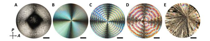
Polarizing Optical Microscopy (POM) images of CNC, TA/CNC, and TA films. POM images of films formed from (A) a CNC suspension; (B to D) TA/CNC suspensions with (left to right) R of 4.0, 5.0, and 6.0; and (E) a TA solution. Films were formed at 22°C and RH = 23%. The concentration of CNCs in (A) to (D) was 3 wt %, and the concentration of TA solution in (E) was 11.3 wt % (750 mM). All films were dried for 24 hours. Scale bars, 420  $\mu$ m. Credit: Science Advances, doi: 10.1126/sciadv.abe3801
