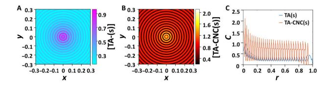
Numerical simulations of ring pattern formation. (A) Spatial distribution of TA-(s), (B) spatial distribution of CNCs, and (C) concentration profiles of TA and CNCs in alternating ring-type bands. In the simulations, the following parameters were used: DA = 10-1, DB = 10-2, DD = 10-2, DE = 10-4,  $d^* = 0.8$ , and  $e^* = 0.2$ . The grid spacing ( $\Delta r$ ) and time step ( $\Delta t$ ) in the numerical simulations were 10-3 and  $1.8 \times 10-8$ . All parameters and variables are in
