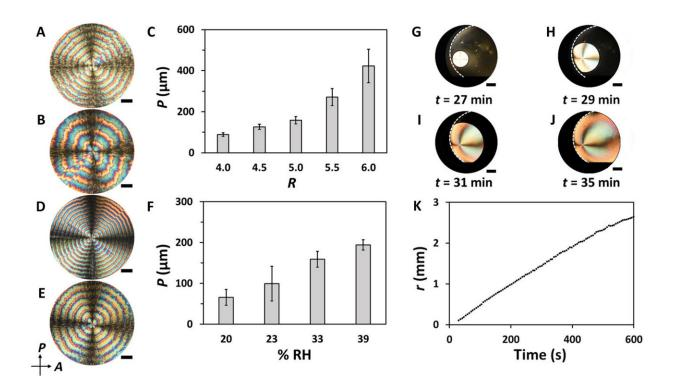
Characterization of ring patterns in TA/CNC films. (A and B) POM images of films formed at R of 4.5 (A) and 5.5 (B). (C) Variation in the average period, P, of the ring pattern, plotted as a function of R. In (A) to (C), films were formed at RH = 33%. (D and E) POM images of films formed at RH = 23% (D) and 33%
