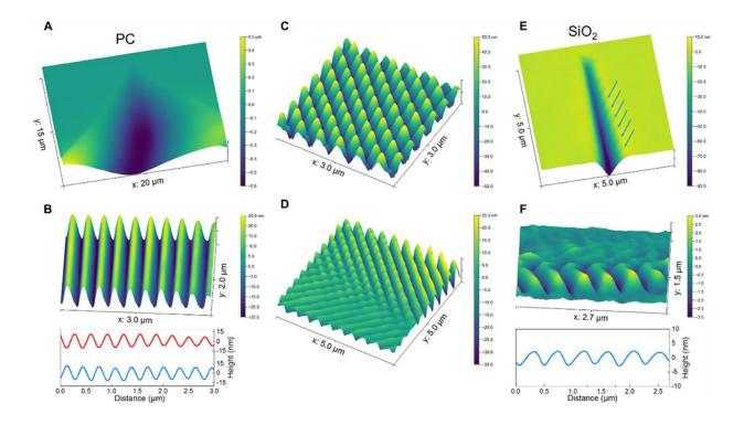
Fig. 3. Cavitation-induced nanostructured fracture surface patterns in polymer and silica glasses. Credit: Institute of Physics
