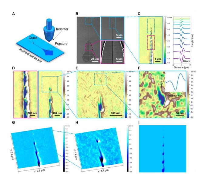
Fig. 1. Observation of the cavitation-dominated crack propagation in a metallic glass. Credit: Institute of Physics
