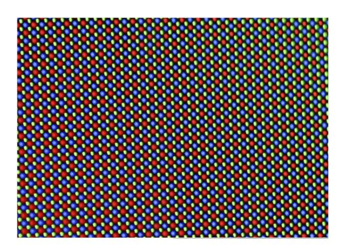
An array of multi-colored LEDs periodically arranged to give off visible light; a combination of InGaN based red, blue, and green LEDs is essential to cover lighting demands efficiently. Credit: Singapore-MIT Alliance for Research and Technology (SMART)
