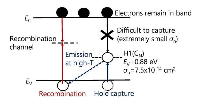
At low temperatures, holes are trapped in H1 and take long to recombine with electrons in EC due to difficulty in electron capture. At high temperatures, the holes escape to EV and recombine with electrons through the recombination channel. Credit: Masashi Kato from Nagoya Institute of Technology
