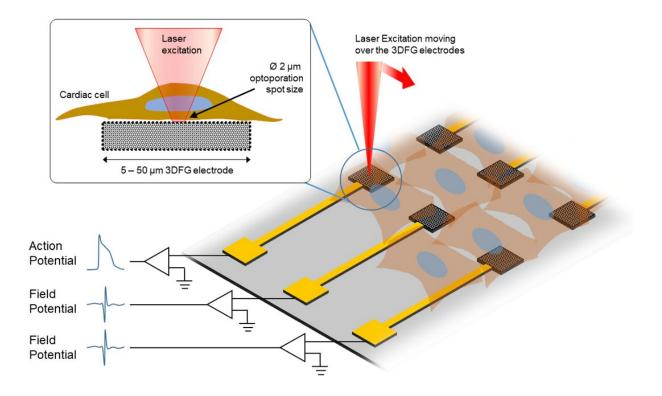
This sketch displays the experimental procedure of ultra-fast laser moving over the 3DFG electrodes. Credit: College of Engineering, Carnegie Mellon University
