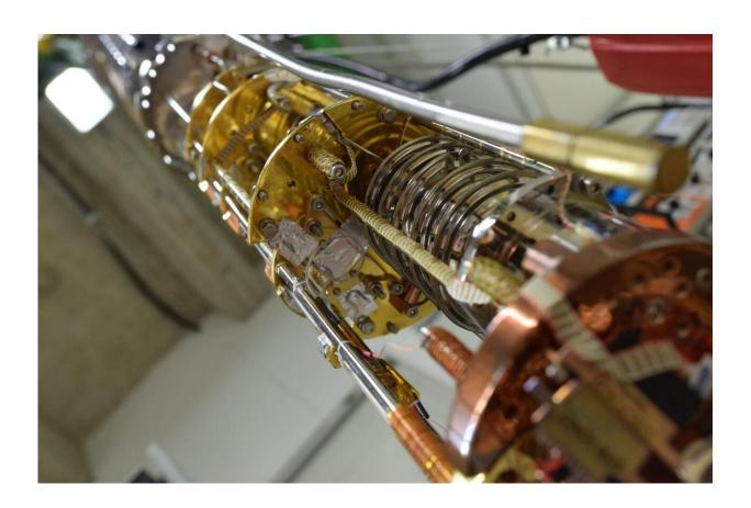
Using a <sup>3</sup>He-<sup>4</sup>He dilution refrigerator, microwave experiments can be performed at extremely low temperatures: a few hundredths of a degree above absolute zero. Credit: University of Stuttgart, Constantin Dressel
