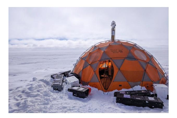
During 2019 field tests near Greenland's Summit Station, a high-elevation remote observing station, the WATSON instrument is put through its paces to seek out signs of life, or biosignatures, 360 feet (110 meters) down a borehole. The winch that holds the drill pokes out the top of the drill tent. Credit: NASA/JPL-Caltech
