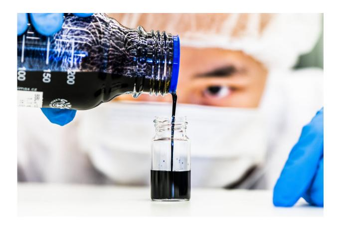
Researchers at Linköping University, Sweden, have developed a stable high-conductivity polymer ink. The new n-type material comes in the form of ink with ethanol as the solvent. Credit: Thor Balkhed
