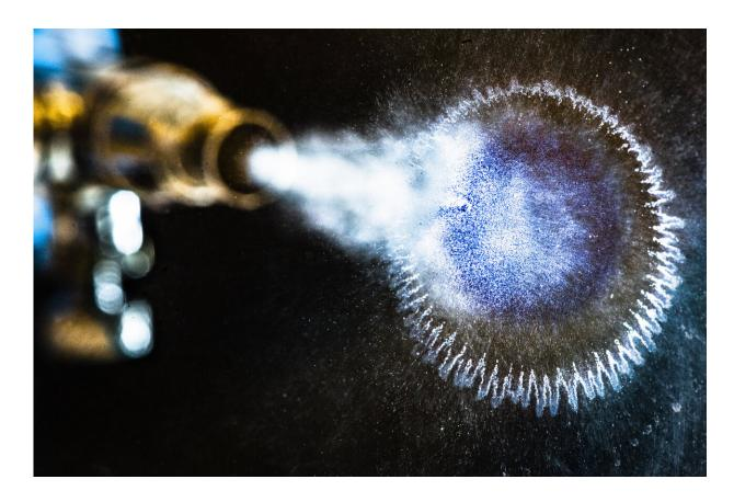
Researchers at Linköping University, Sweden, have developed a stable high-conductivity polymer ink. The ink can be deposited by simply spraying the solution onto a surface, making organic electronic devices easier and cheaper to manufacture. Credit: Thor Balkhed
