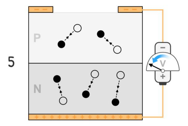
5. The bias voltage is then lowered, "quenching" the semiconductor to remove the existing carrier pairs. Credit: Sean Kelley/NIST
