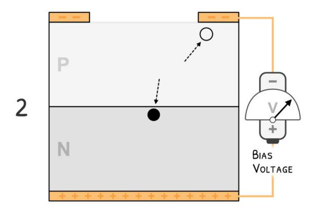
2. The electron and hole are accelerated by the applied bias voltage. Credit: Sean Kelley/NIST
