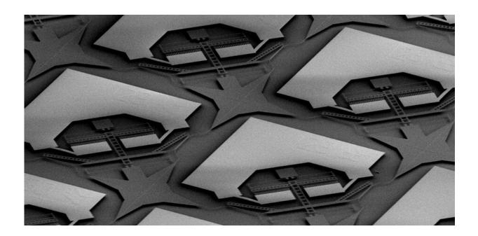
Partial SEM image of the switch matrix: the whole structure patterned in the top silicon layer by dry etching seems to "float" as the oxide is removed. Each matrix unit contains an electrostatic comb drive that can selectively move portions of the waveguides to establish a desired light path from one of the 32 input ports to one of the 32 output ports. Credit: Han et al.
