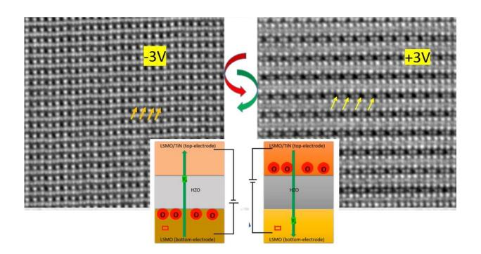
Electron microscope images, in the left panel a sample with a lot of oxygen atoms (some indicated with arrows), in the right panel a sample with many oxygen vacancies (some indicated with arrows). The schematic illustration shows the movement of oxygen atoms and oxygen vacancies for two settings of the electric field over the capacitor. Credit: Nukala et al. / University of Groningen
