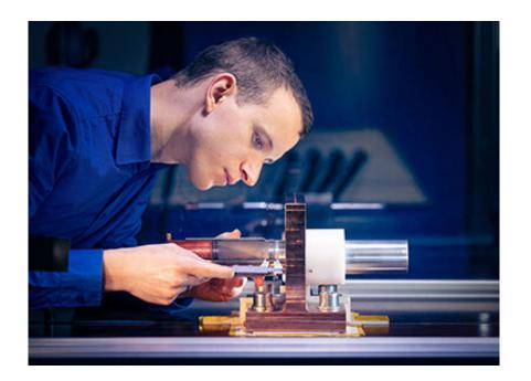
With magnetic pulse welding, the magnetic pressure of a tool coil ensures a highspeed collision and the formation of a solid state joint of several millimeters in width, as well as high stability and leak tightness, even under extreme application conditions. Credit: ronaldbonss.com
