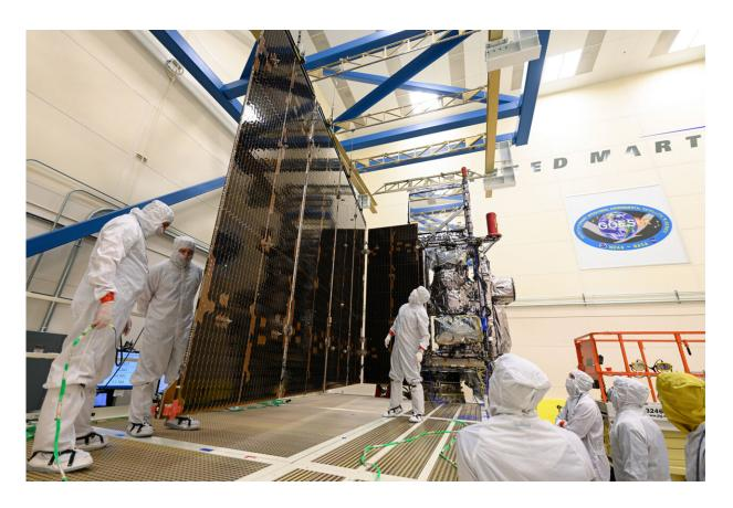
Engineers conduct the GOES-T solar array deployment test. Credit: Lockheed Martin
