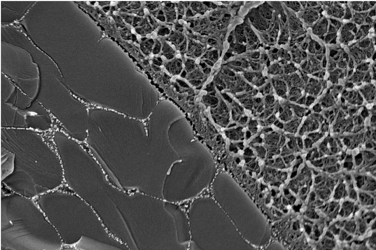
The interface between the hydrogel (left-hand side) and the PDMS (on the right-hand side). The images was taken at 100,000 times magnification. Credit: University of Leeds
