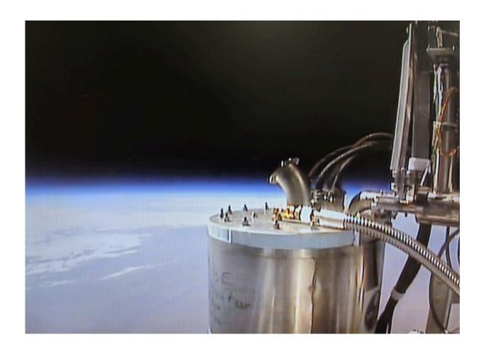
This image shows BOBCAT hardware used to demonstrate the successful transfer of cryogenic fluids into a dewar during a balloon demonstration in August 2019. The shot was taken when the balloon reached its float altitude of 133,000 feet. Credit: NASA
