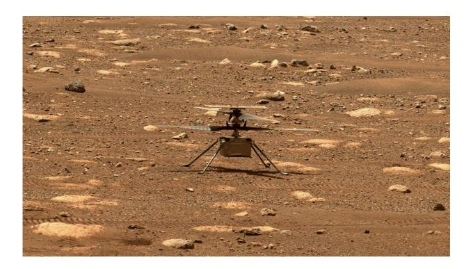
NASA's Ingenuity helicopter unlocked its blades, allowing them to spin freely, on April 7, 2021, the 47th Martian day, or sol, of the mission. This image was captured by the Mastcam-Z imager aboard NASA's Perseverance Mars rover on the following sol, April 8, 2021. Credit: NASA/JPL-Caltech
