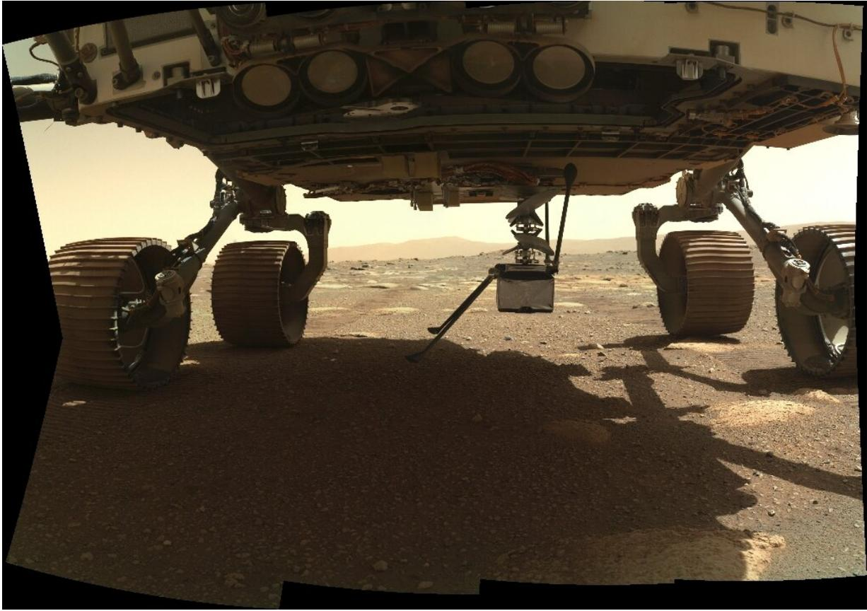
Ingenuity is now alone on the surface of Mars after detaching from the belly of the Perseverance rover
