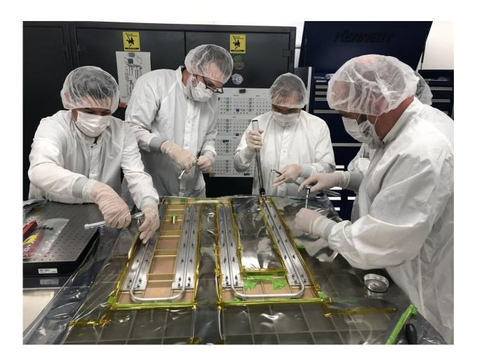
Technicians and engineers at NASA's Jet Propulsion Laboratory work together on Sept. 12, 2019, to bond thermal tubing to a panel built for NASA's Europa
