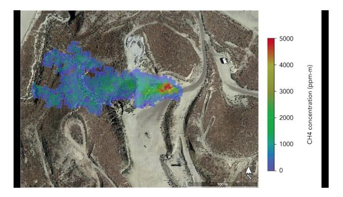
A methane plume detected by NASA's AVIRIS-NG in summer 2020 indicates a leaking gas line in oil field in California. The operator subsequently confirmed and repaired the leak. Credit: NASA/JPL-Caltech
