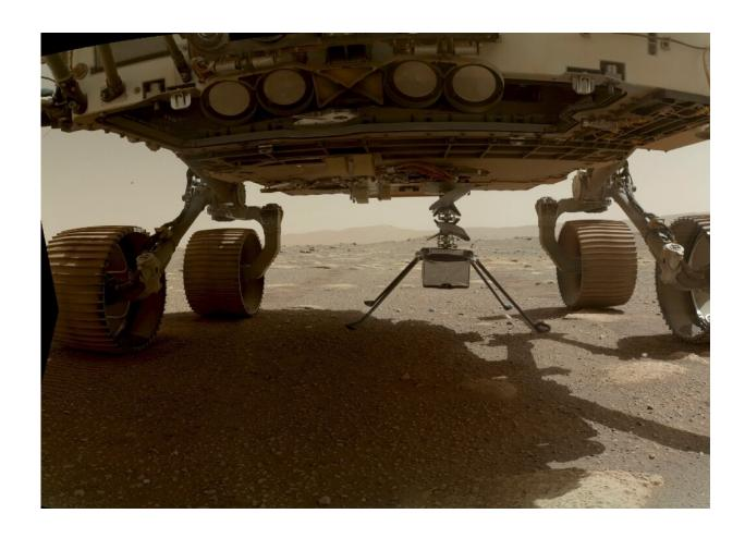
NASA's Ingenuity Mars Helicopter, with all four of its legs deployed, is pictured before dropping from the belly of the Perseverance rover in March 2021
