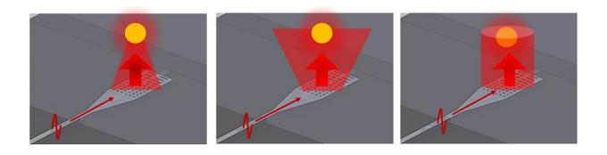
Schematic of three different nano flashlights for the generation of, left to right, focused, wide-spanning, and collimated beams. Each could have different applications. Credit: Robin Singh
