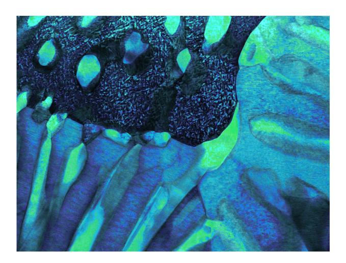
ORNL researchers used electron beam powder bed fusion to produce refractory metal molybdenum, which remained crack free and dense, proving its viability for additive manufacturing applications. Credit: ORNL/U.S. Dept. of Energy
