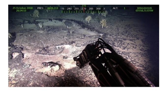
Manipulator arm on the HyBIS hybrid remotely operated vehicle collecting crust samples from the Rio Grande Rise. Credit: Bramley Murton
