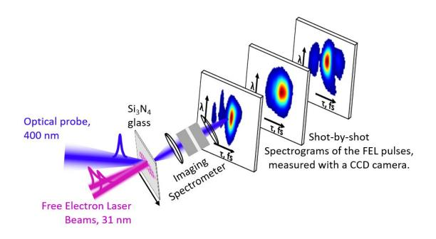
An optical shutter created by ionization allows an ordinary camera to measure a femtosecond pulse from a free electron laser. Credit: Los Alamos National Laboratory
