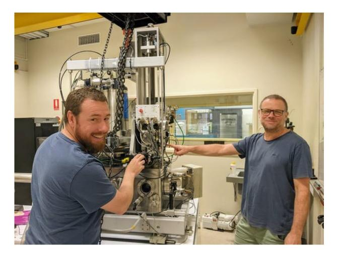
Chris Kirkland (left) and Tim Johnson loading samples into a secondary-ion mass spectrometer, which shoots a beam of ions into zircon crystals to determine their age and oxygen isotope composition. Credit: The Conversation
