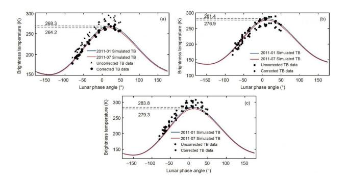
Average microwave TB simulation and data. (a) 89GHz; (b) 157GHz; (c) 183GHz. Credit: Science China Press
