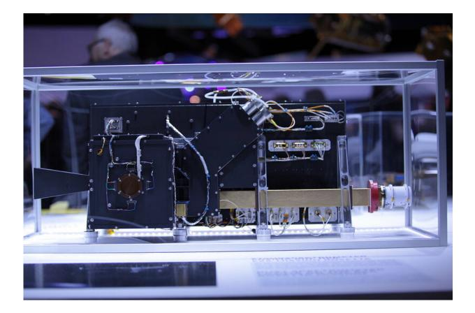
COSIMA is the in-situ dust analyzing instrument on board space probe Rosetta to comet 67P/Churyumov-Gerasimenko. Credit: DLR German Aerospace Center, licensed under CC BY 2.0
