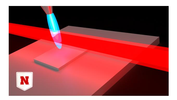
A rendering of an infrared laser striking a flame. Husker researchers have shown how a laser can modify chemical reactions taking place within a flame, allowing them to coat materials with performance-enhancing chemicals while avoiding a side effect that complicates the construction of semiconductors and other microelectronic components. Credit: Scott Schrage | University Communication
