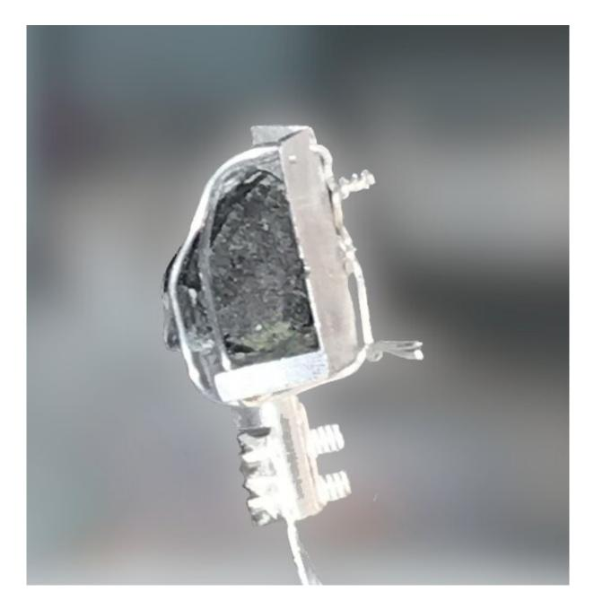
The researchers' measurements were made on a high-quality single crystal of potassium copper fluoride. The neutrons scatter from the quantum spins of the copper sites. The scattering is then analyzed to extract the spin transport along the chains. Credit: Oak Ridge National Laboratory, U.S. Dept. of Energy.
