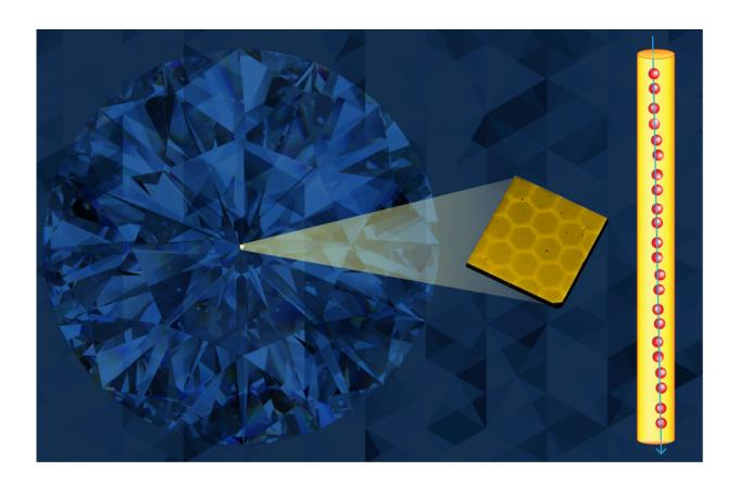
Ion beams can create chains of closely coupled quantum bits (qubits) based on nitrogen-vacancy "color centers" in diamond for use in quantum computing hardware. The honeycomb pattern in the photo shows the difference between areas exposed to the beam (darker) and masked-off areas. Results indicate it should be possible to create 10,000 coupled qubits over a distance of about the width of a human hair, an unrivaled number and density of qubits. Credit: Susan Brand/Berkeley Lab
