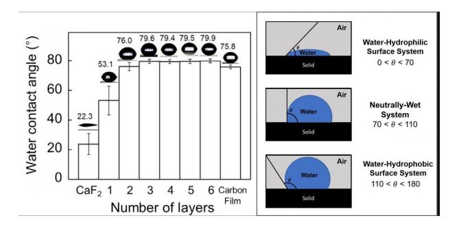
Macroscopic observation of WCA shows that increasing the number of graphene layers results in higher WCA, which hints hydrophobicity of multilayer graphene. Credit: Institute for Basic Science
