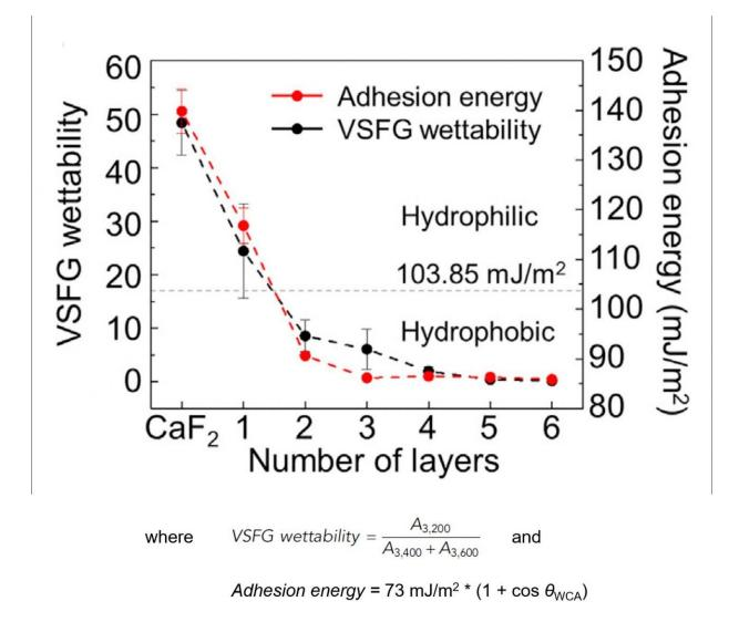
The calculated VSFG wettability is plotted against adhesion energy from macroscopic observation of WCA. Both values coincide closely and indicate increasing hydrophobicity as the number of graphene layers increases. Credit: Institute for Basic Science
