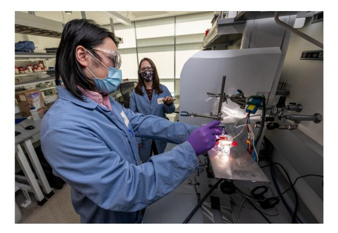
Guosong Zeng, a postdoctoral scholar, and Francesca Toma, a staff scientist, both in Berkeley Lab's Chemical Sciences Division, test an artificial photosynthesis device made of gallium nitride. Rather than degrading over time, which is typical for devices that turn water and light into hydrogen fuel, Toma and Zeng discovered that this device improves. Credit: Thor Swift/Berkeley Lab
