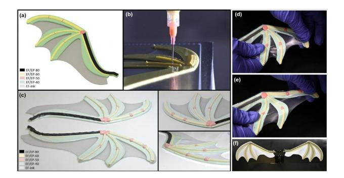
(a) Illustration of the structural design. (b) Direct-ink-writing of the hybrid structure. (c) Cured structure (area of ~90 cm<sup>2</sup> per wing, membrane thickness ~0.7 mm, total arm thickness ~3.5 mm). (d) Flexibility and cohesiveness of the wing structure under small strains. (e) Flexibility and cohesiveness of the wing structure under large strains. (f) Wings mounted on actuation mechanism. Credit: SUTD
