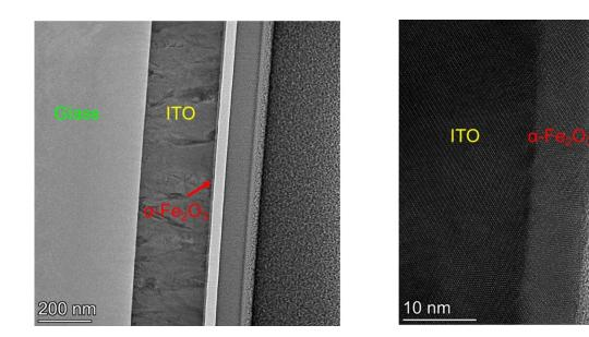
Rust would be an extremely cheap and stable photoelectrode material to produce green hydrogen with light. But the efficiency is limited. The TEM image shows a photoanode containing a thin photoactive layer of rust. Credit: Technion
