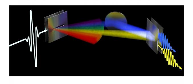
Representation of a transmitter (left) broadcasting a signal with strong angular dispersion. Each frequency is represented by a different color and comes out in a different direction, which produces a rainbowlike structure. Two of the frequencies make it to the receiver (right), one represented by yellow (LOS path) and another by blue (NLOS path incorporating a reflection off a surface). Credit: Mittleman Lab, Brown University
