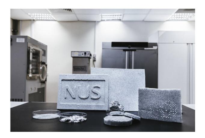
These metal-based aerogels have high thermal and mechanical stability, and they could potentially be used as light-weight building materials and for growing cells for biomedical purposes. Credit: National University of Singapore
