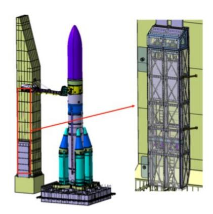
Pyrotechnic actuators detonate to burst hinges open allowing the umbilicals to
