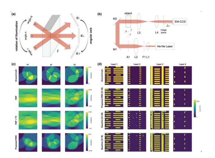
(a) A schematic on the limited-angle tomography. Each illumination angle in an angular axis corresponds to a time step in an analogous temporal axis. (b) An optical apparatus used for experiments under the strong scattering condition. (c) Qualitative comparison on reconstructions of conventional inverse algorithms (FBP: filtered backprojection, FBP + TV: TV-regularized filtered
