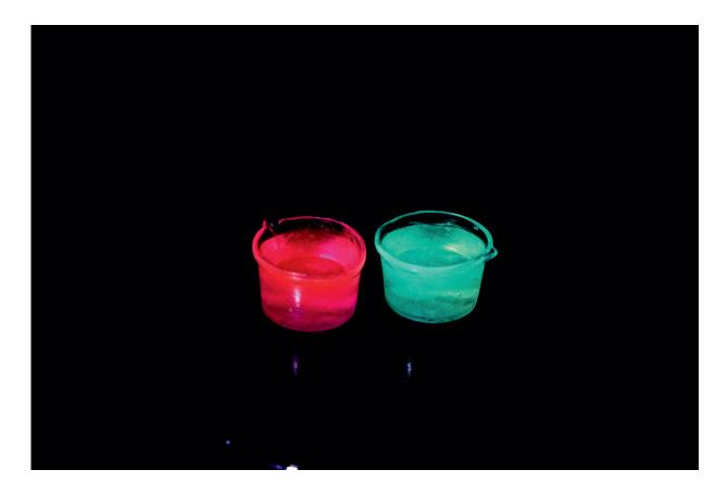
Injection molding of the newly developed Glassomer composite enables the production of transparent fused silica beakers. The beakers are filled with dyed water or fluorescent liquids. Credit: Glassomer GmbH
