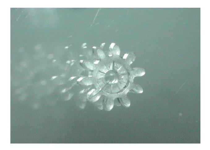
Transparent fused silica gears produced by injection molding of the newly developed Glassomer composite. Credit: Glassomer GmbH
