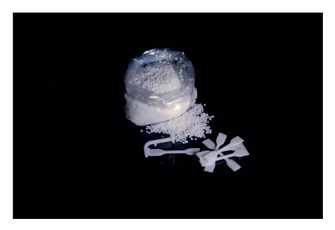
Glassomer injection molding granules and injection molded structures. Credit: Glassomer GmbH
