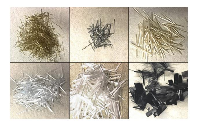
ORNL researchers used fiber reinforcements made of steel, glass and carbon to develop a concrete mix that demonstrated high early strength within six hours of production, which is needed for the precast concrete industry. Credit: ORNL/U.S. Dept. of Energy
