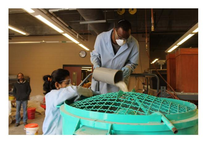
Researchers from ORNL and the University of Tennessee collaborated to perform lab-scale evaluations on the high early strength fiber-reinforced self-compacting concrete mix. Credit: University of Tennessee
