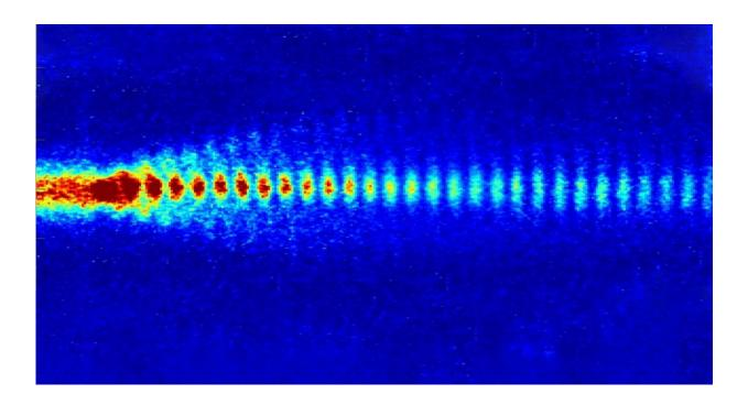
A train of short proton bunches travels through the plasma field, forming a wave on which electrons can be accelerated. Credit: AWAKE
