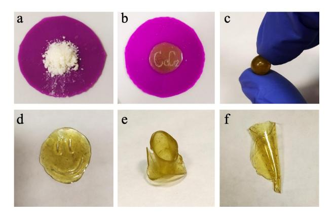
Mechanical treatment of mitranol-based polymers: a - primary polymer as white powder; b - melted polymer, c-f - various forms of the polymer after being melted repeatedly. Credit: SPbU
