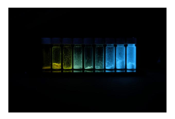
These polymers, seen here under UV light, are composed of the exact same components. The only difference is their chain length. Credit: Suiying Ye / ETH Zurich
