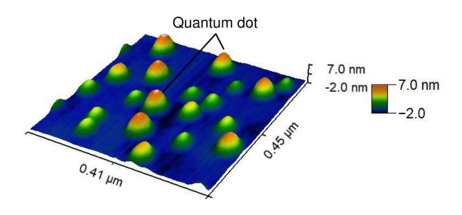
The quantum dots in the opto-spintronic nanostructure are made from indium arsenide (InAs). Each quantum dot is around 10,000 times smaller than the thickness of a human hair. Credit: Yuqing Huang
