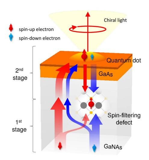
In the opto-spintronic nanostructure, an electron spin polarisation degree greater than 90% is achieved at room temperature in a quantum dot, via remote defectenabled spin filtering through an adjacent layer of gallium nitrogen arsenide (GaNAs). When such a spin polarised electron recombines, it emits chiral light. The spin state of the electron determines whether the electromagnetic field of
