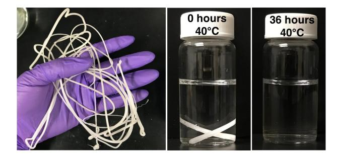
A melt-extruded PCL (polycaprolactone) plastic filament (left) with embedded nanoclusters of the enzyme lipase enshrouded with RHP degraded nearly completely into small molecules within 36 hours in warm (104 F) water. Credit: Christopher DelRe, UC Berkeley
